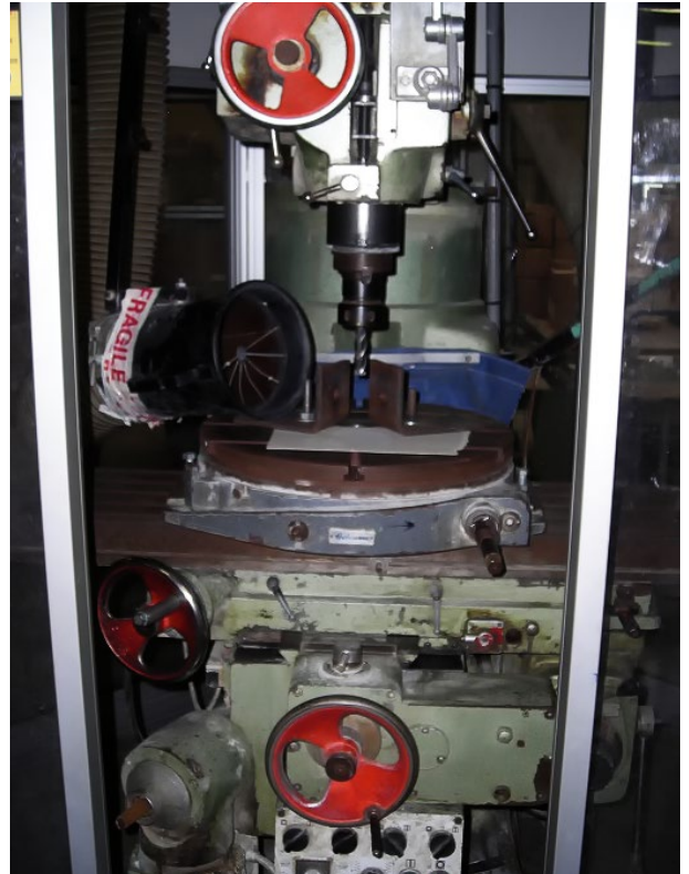
Drill with limited dust control
