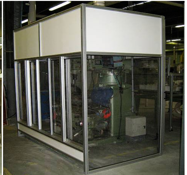
Router fully enclosed
