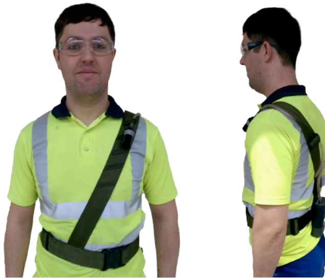
Fig. 1 & 2: Personal air sampling unit for airborne fibres
