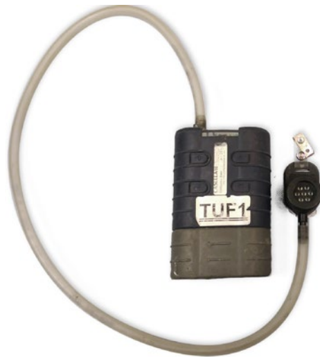
Fig. 3: Sampling assembly UKEA head (total dust)
