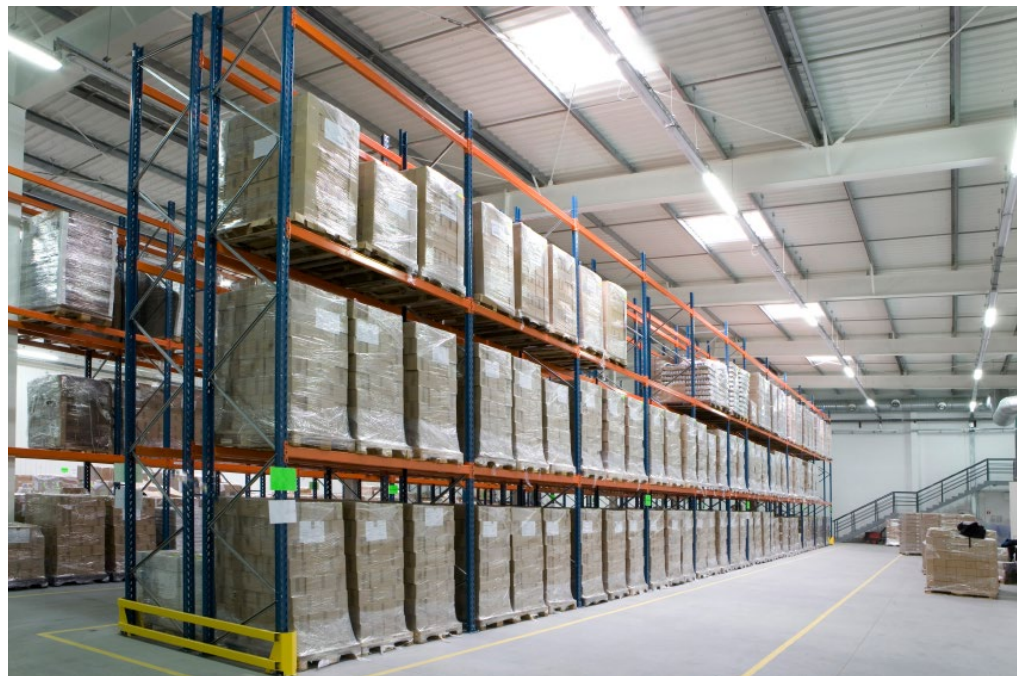
Example of pallet racking
