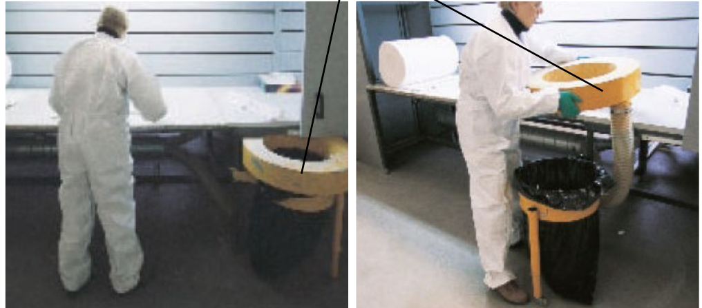
Fig. 3+4: Bin for off-cuts in finishing tasks. In case of handling ASW/RCF person needs to wear a mask (appropriate PPE).
