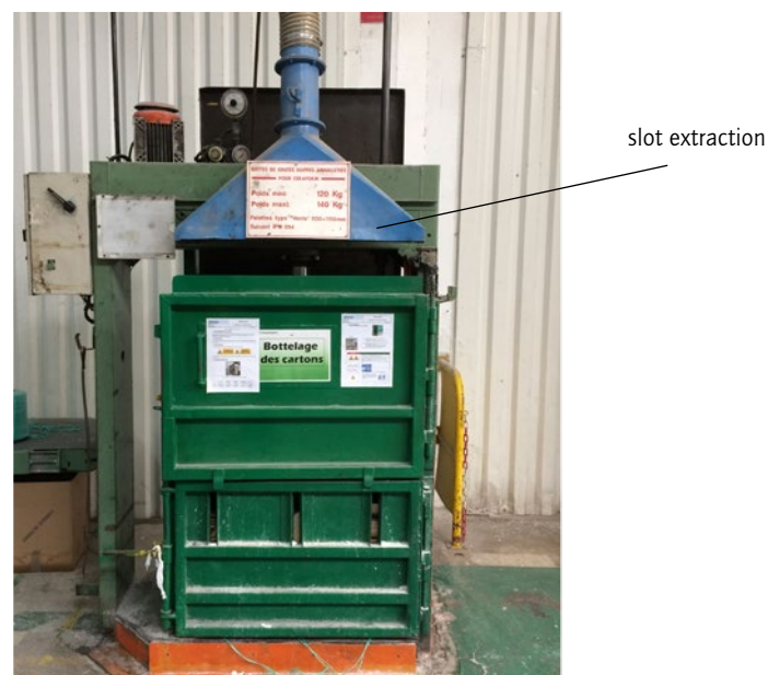
Fig. 2: Press for empty bags with LEV capture device (slot extraction) linked to LEV system
